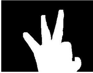
Fig.4. Output after dilation and erosion.
